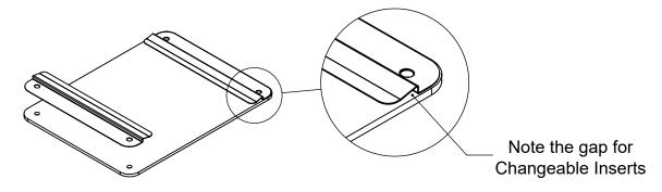
Step 3: Attach both Hinges to the left or right side of the Glassboard as shown. Securely tighten the Screw and Lock Nut using the provided 1/4" Allen Wrench and a 1/2" Socket wrench.
