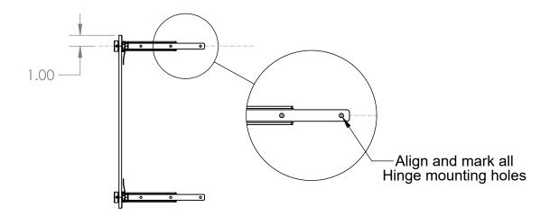
**Installation Step B:** When installing into studs, drill a 7/64" pilot hole using a straight bit for the Self-Tapping Screws. If wall studs are not available, drill a 1/4" hole to mount Wall Anchors.
