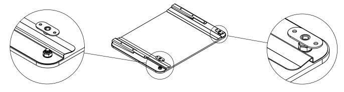
**Step 6:** Flip the Glassboard to allow access to the front face. On each Screws add one Standoff Cap and secure by tightening the side Set Screws with the provided 2mm Allen Wrench.
