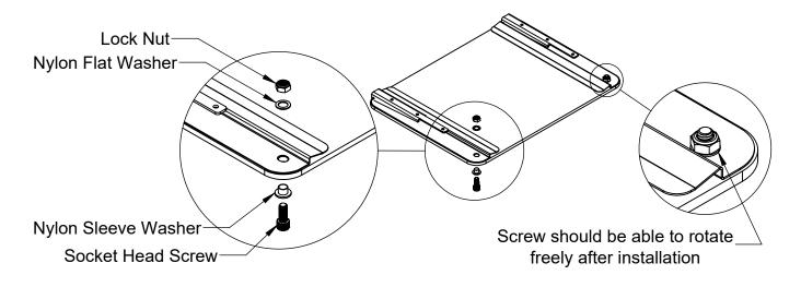
**Step 5:** Attach the Wall Catch to the Screws installed in Step 4, and align parallel to the Tracks.
