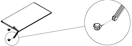
Step 4: Remove the side mounted feet using a 5/32" Allen wrench.
