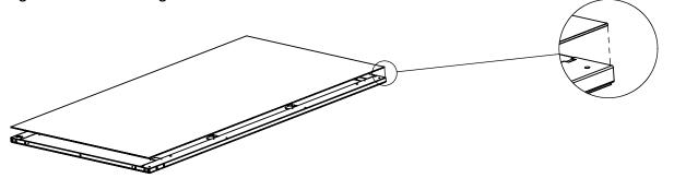
**Step 7:** (Optional) If the glassboard has a rear magnetic panel pry one corner away from the glass using a putty knife. Continue to separate the magnetic panel from the glassboard until fully separated.
