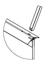
**Step 3:** Use the included wrench to tighten the socket screw. The screw must be completely tightened for a secure leg connection.
