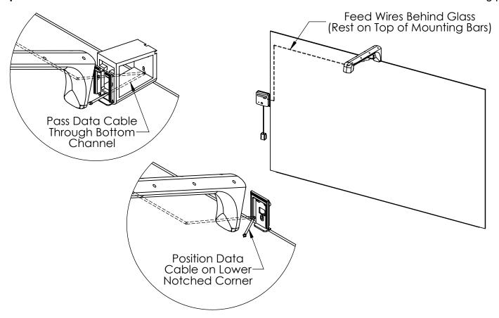
**Step 4:** Push the Control Pad onto the mounting plate. Plug in the Power Adapter to outlet if using Wi-Fi, or if power is not supplied by Ethernet connection. Hide wires behind Glassboard and use Wire Clips. Use provided screws to support clips.
