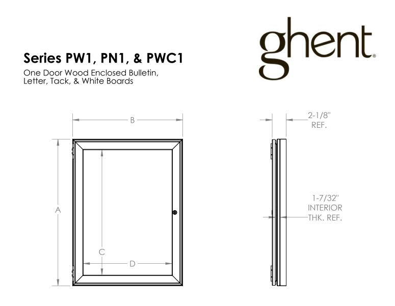
Walnut framing shall be stained first and then clear-coated. Oak framing shall be clearcoated only. Door shall be 1/8" acrylic. Door to be equippped with nickel hinges and built-in lock with keys. The back panel of the case shall be fitted with optional vinyl, cork, tackboard, Porcelain, or changeable letterpanels for interior use. Available Sizes:
