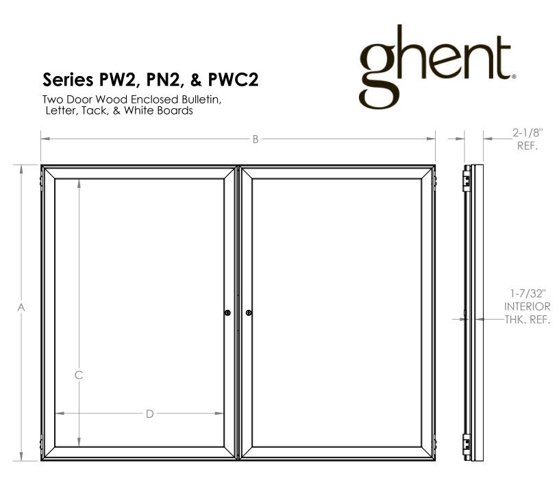
Walnut framing shall be stained first and then clear-coated. Oak framing shall be clearcoated only. Door shall be 1/8" acrylic. Door to be equippped with nickel hinges and built-in lock with keys. The back panel of the case shall be fitted with optional vinyl, cork, tackboard, Porcelain, or changeable letterpanels for interior use. Available Sizes:
