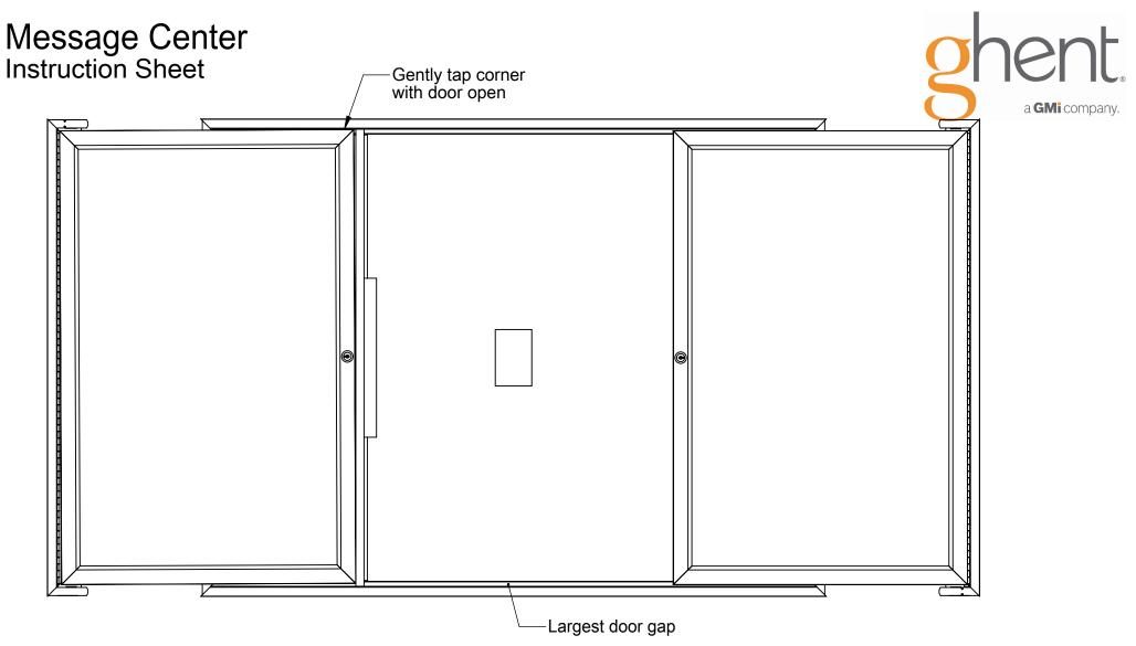
Your new Ghent Message Center has been assembled and inspected to Ghent's high quality standards. Occasionally during shipment, your message center's door(s) may shift. This shift results in an uneven gap between the door(s) and the body of your unit.
