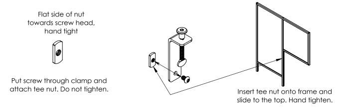
Step 3: Pre-assemble screw and tee nut onto foot as shown, slide foot onto frame and hand tighten.
