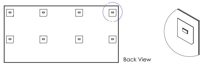
Step 2: Remove the cleat system from the Define unit.
