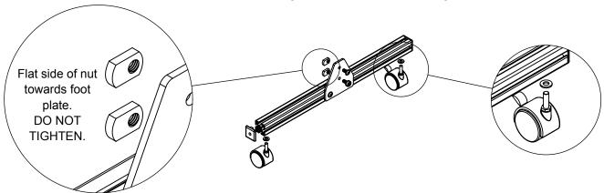
**Step 4:** Install the foot assembly onto the clear panel as shown, tighten hardware accordingly. Repeat on other side.
