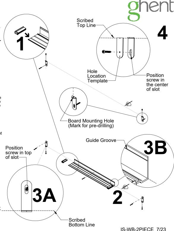
**STEP 5**: Slide the TOP L hangers UP until the screw is resting in the lower end of the L hanger's slot. Lift the **LEFT** board onto the premounted tray/L hangers.
