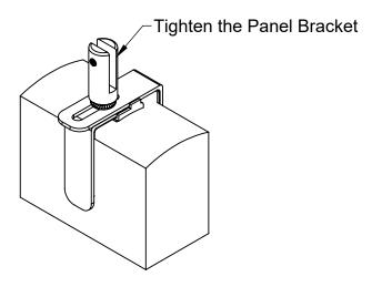
**Step 5:** Slide the acrylic panel into the panel bracket. Secure the panel by tightening the set screw in the panel bracket with the provided Allen wrench.
